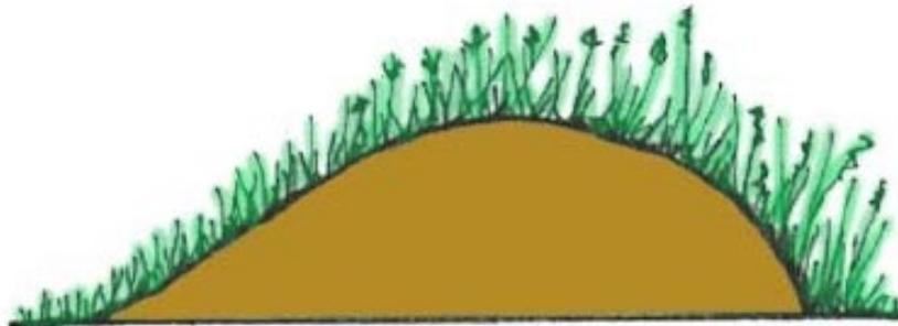
desirable shape for a berm
