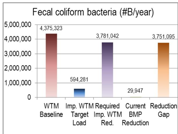
**Figure 4-3. Comparisons of WTM baseline loads, implementation target load, required implementation load reduction, load reduction from current BMPs, and reduction gap for the Anacostia River watershed.**
