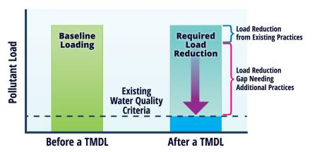
A TMDL identifies the maximum amount of pollutant load that the water body can receive and still meet water quality criteria. The green bar on the left represents the current pollutant load (sometimes called the baseline) that exists in a water body before a TMDL is developed. The elevated load causes the water body to exceed water quality criteria. The blue bar on the right shows the amount that the pollutant load will need to be reduced for the water body to meet water quality criteria.
