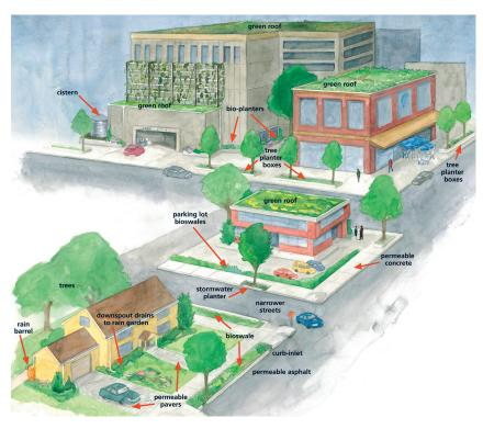
Conceptual city block with various stormwater management practices. Rain barrels, permeable pavers, bioswales and other water-friendly options will be used throughout the County to improve water quality. Credit: U.S. Environmental Protection Agency; Office of Wetlands, Oceans and Watersheds
